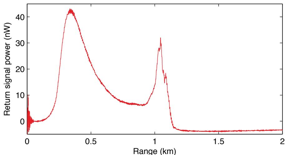
Figure 5. Return signal measured during lidar field test. The instrument was directed at an elevation of  $20^\circ$  to the horizontal. The signal around 1 km is due to cloud. The transmit pulse energy was 0.39 mJ.
