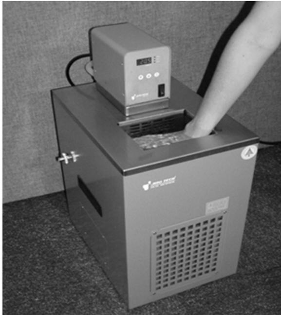
FIG. 2. Cold Pressor used in the pain experiments.
