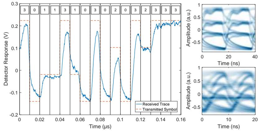
Fig. 3. Received 4-PAM optical signal at 100 MSamples/s, with the transmitted symbol. To the right are the eye diagrams for 50 MSamples/s (upper) and 100 MSamples/s (lower) symbol rates.
