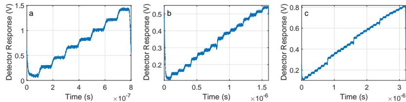
Fig. 6. Levels used for generating OFDM signals with a) 3, b) 4 and c) 5 bit resolution using array B. Symbols were transmitted sequentially at a rate of 10 MHz.
