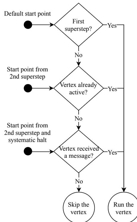
Figure 4: Execution flow of the vertex selection mechanism
