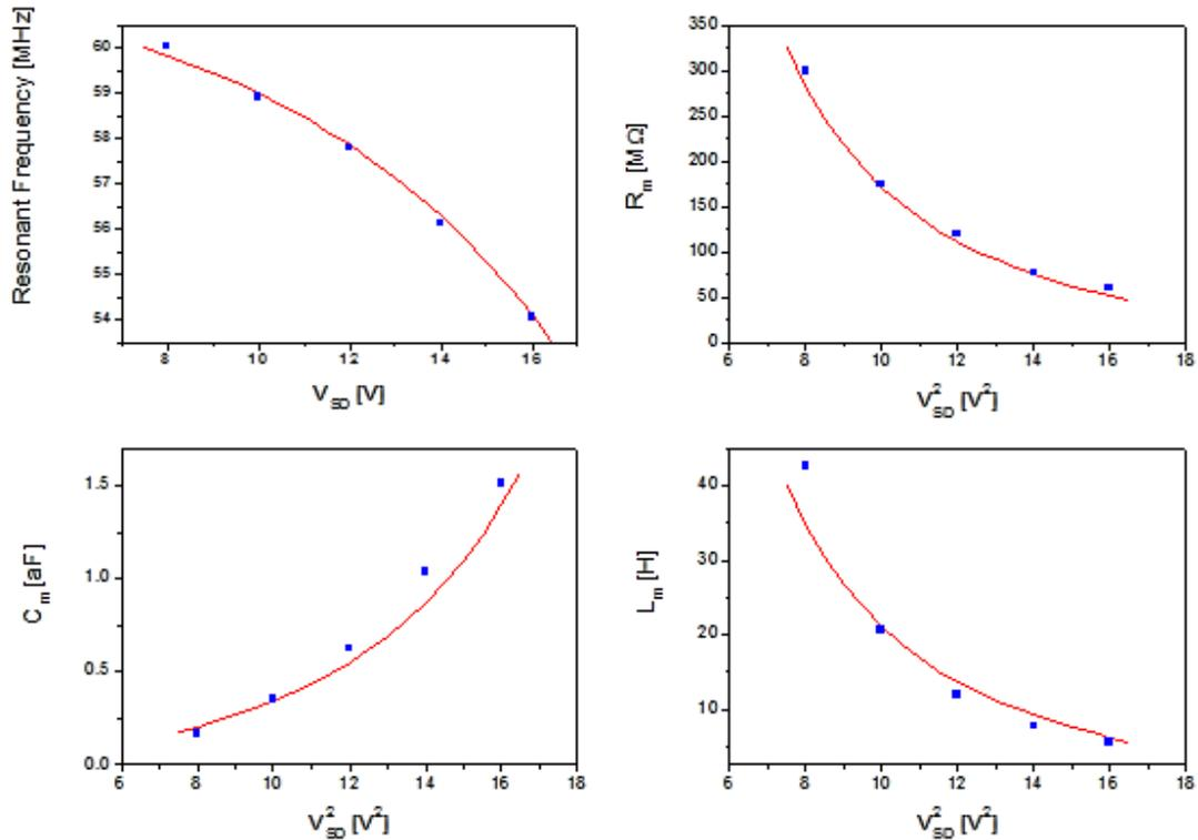
**Figure 4.** Comparison of the small signal nanotube resonator model to the experimental results. The device geometry was estimated from SEM images. Squares (blue) are measurements and the red lines are theoretical predictions obtained with CNF Young's modulus  $E=0.41$  TPa,  $C_{D0}=4.5$  aF and  $Q_0=47$ .
