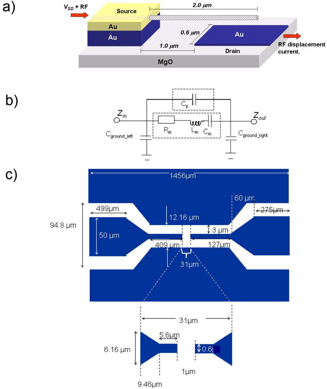
**Figure 1.** (a) Schematic drawing of two-terminal CNF relay. (b) Equivalent circuit (c) Substrate layout, designed to reduce parasitic capacitance. Note, drawing is not to scale.
