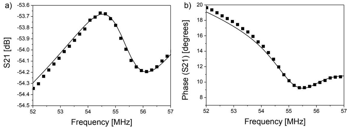
**Figure 3.** (a) Amplitude  $S_{21}$  and (b) phase for the high frequency resonance with  $V_{SD} = 17\text{V}$ . The experimental data is shown as square symbols. The full lines are obtained from assuming small signal model behaviour and simulating the entire system in the ADS circuit simulator. By fitting the model to the experimental data it is possible to extract the motional impedance parameters,  $R_m$ ,  $C_m$  and  $L_m$ .
