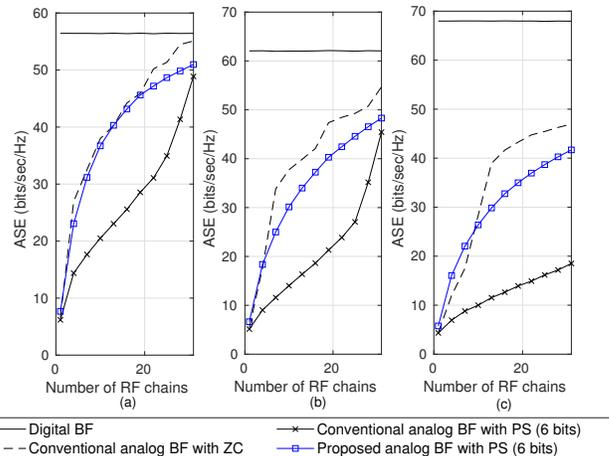
Fig. 3. ASE as a function of the number of RF chains  $M_R$  for  $T = 40$ ,  $N_p = 6$ ,  $N_T = 16$  and  $\text{SNR} = 15\text{dB}$ . (a)  $N_R = 32$ ,  $M_R^e = 32$ , (b)  $N_R = 64$ ,  $M_R^e = 32$ , and (c)  $N_T = 128$ ,  $M_R^e = 64$ ,
