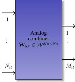
Fig. 1. Block diagram of the conventional analog combiner [4] used for wideband mmWave MIMO channel estimation with HBF reception. The combiner connects via phase shifters its  $N_R$  inputs from the respective RX antennas to the  $M_R$  receive RF chains.
