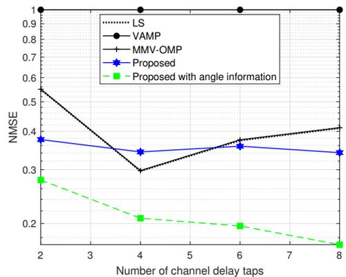
Fig. 8. NMSE performance as a function of the number of the channel delay taps  $L$  for  $N_T = 8$ ,  $N_R = 32$ ,  $M_R = 4$ ,  $M_R^e = 32$ ,  $N_p = 6$ ,  $T = 20$ , and  $\text{SNR} = 15\text{dB}$ .
