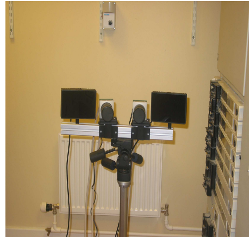
Fig. 1. Stereo rig of the high-speed scanner
