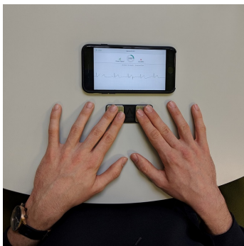
Figure 1: ECG monitor connected to the smartphone application.
