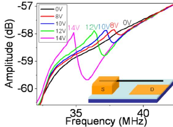
**Figure 4.** High frequency measurement result of cantilever system. The peak of the transmission parameter  $S(21)$  indicates the mechanical resonance of suspended CNT. Inset shows the schematics of device for direct electrical measurement using network analyzer.
