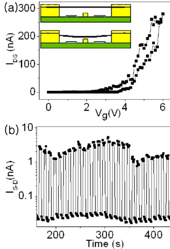
**Figure 5.** The electromechanical properties of doubly clamped CNT based NEM switch. (a)  $I$ - $V_g$  characteristics of doubly clamped system. Inset shows the schematics of doubly clamped CNT based NEM switch before (up) and after (down) actuation. (100mV of Source-drain bias was applied during  $I$ - $V_g$  measurements). (b) The source-drain current monitoring as a function of time during repetitive switching on and off operation.
