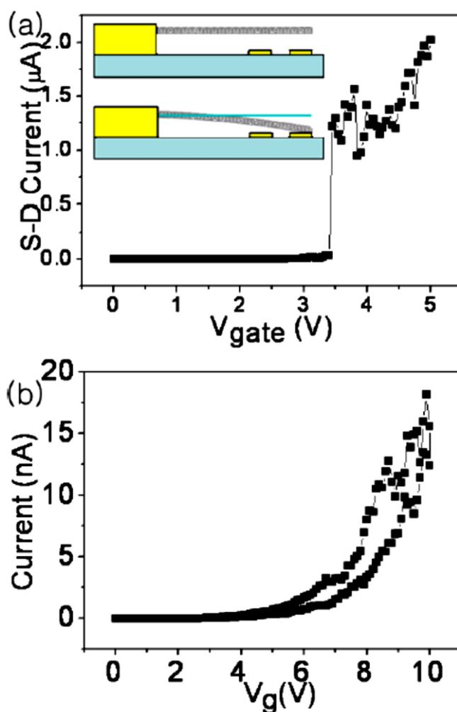
**Figure 3.** The  $I-V_g$  characteristics of cantilever type NEM switch. (a) The step-like current increase was occurred as gate voltage increased. Inset shows the schematics of cantilever type NEM switch before (up) and after (down) actuation. (b) The  $I-V_g$  curve shows relatively slow switch on and off behavior. Theoretically expected hysteresis behavior is found from the gate voltage sweep.
