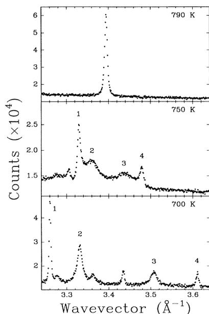
FIG. 1. Neutron powder diffraction spectra well above, close to, and well below  $T_c$  showing the splitting of the hexagonal (202) peak into the (402), (222), (222), and (402) peaks in the monoclinic phase (labeled 1-4, respectively). The lattice melting and subsequent recovery of the Bragg peaks through the transition are apparent.
