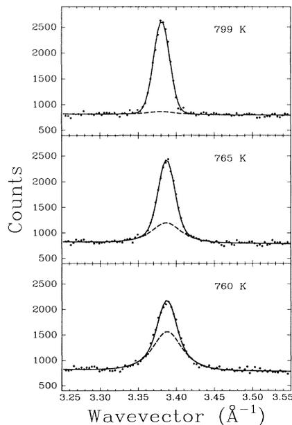
FIG. 3. The temperature evolution of the line profile of the (202) peak above  $T_c$ . The broken line shows the exponential component, and the full line shows the complete analyzed profile with the Bragg component included.
