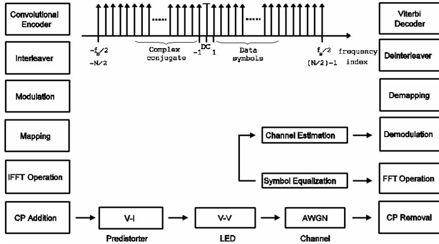
Notes: The LED characteristics are modelled through the V-I block. The predistorter is modelled through the V-V block. IFFT bin assignment.  $f_s$  is the sampling frequency,  $N$  are the number of the IFFT bins (IFFT length or the OFDM
