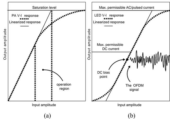
Notes: The non-linear transfer characteristic distorts the OFDM signal in RF as well as in optical applications. Linearisation through predistortion helps to improve system performance.
