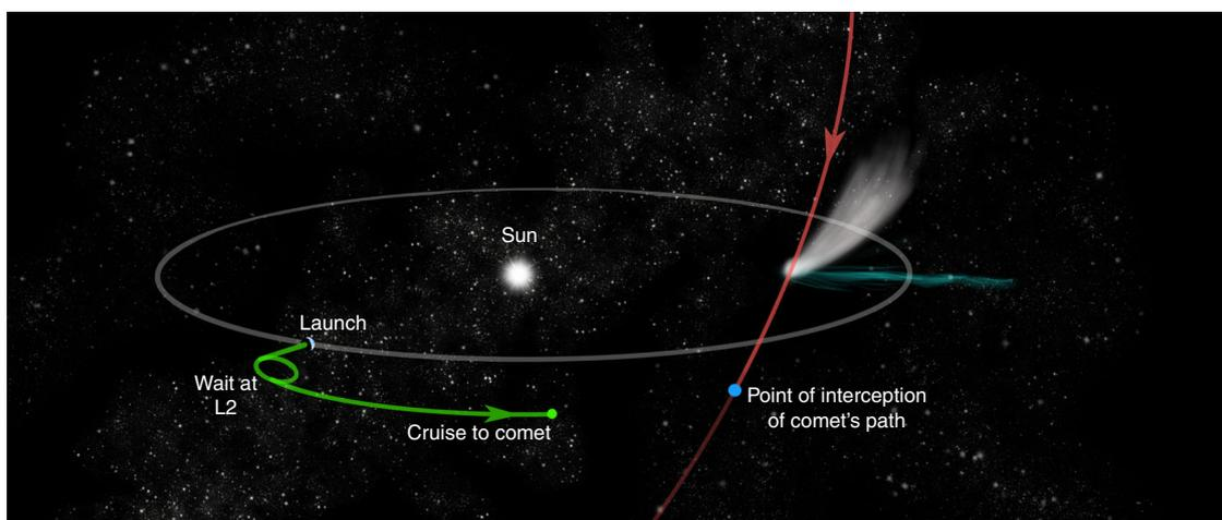
**Fig. 1** Sketch of mission phases. The spacecraft launches from Earth and waits at L2 until a suitable comet is discovered, before departing on an interplanetary cruise to be in the right place at the right time to intercept the comet as it crosses the ecliptic plane. The smaller probes are released just before arriving at the comet. The trajectory of the spacecraft is in green, while the comet’s orbit is in red.
