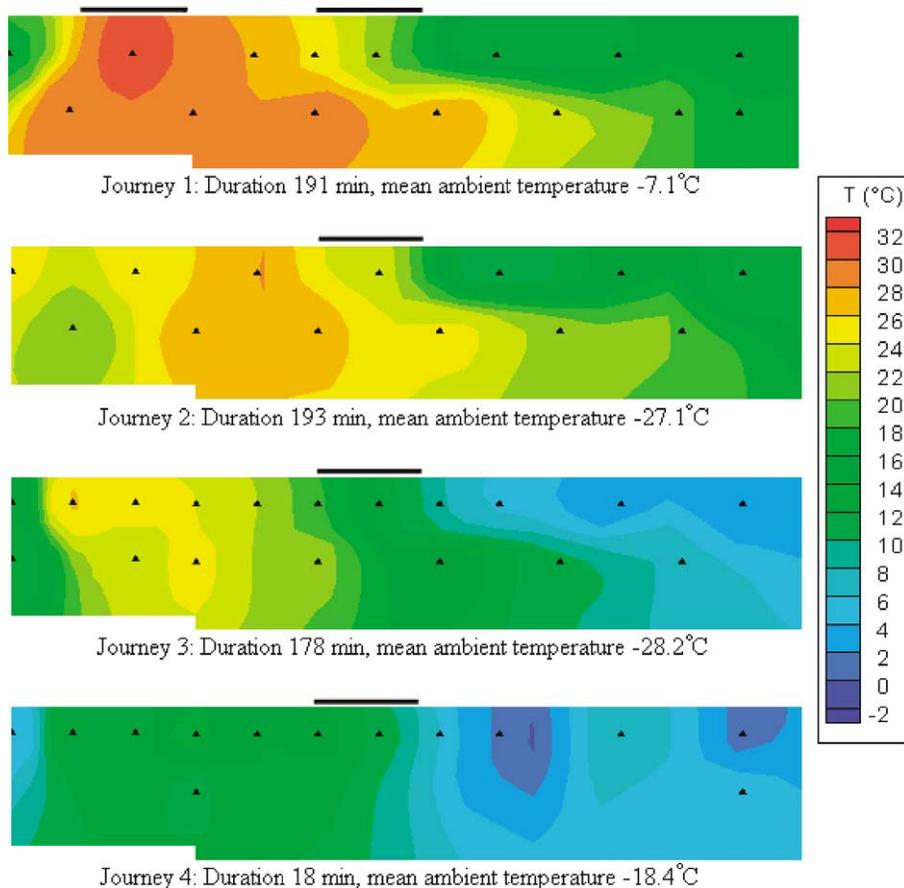
**Fig. 3.** Interpolated temperature variations along the centre of a 16-m trailer during four winter journeys. Dark dashes above each image indicate locations of open air vents. Small black triangles within each image indicate locations of temperature sensors.
