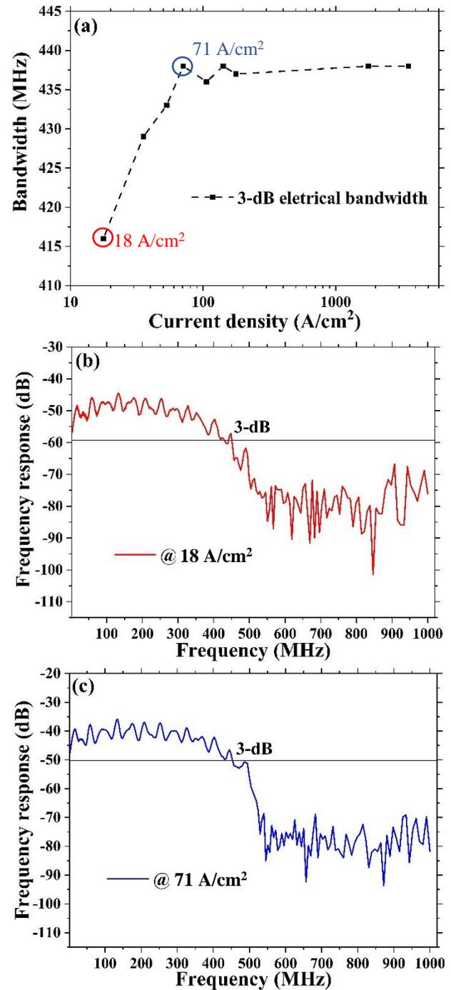
**Fig. 4.** (a) 3-dB electrical modulation bandwidth of the UV-C  $\mu$ LED as a function of current density; small signal frequency responses of the UV-C  $\mu$ LED at (b) 18 and (c)  $71 \text{ A/cm}^2$ .
