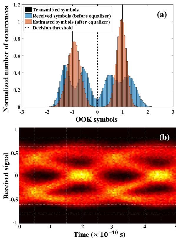
**Fig. 6.** (a) Normalized number of occurrences of transmitted and received symbols assuming the OOK modulation scheme at 800 Mbps and (b) the eye diagram of received symbols assuming the same measurement conditions using the UV-C  $\mu$ LED.
