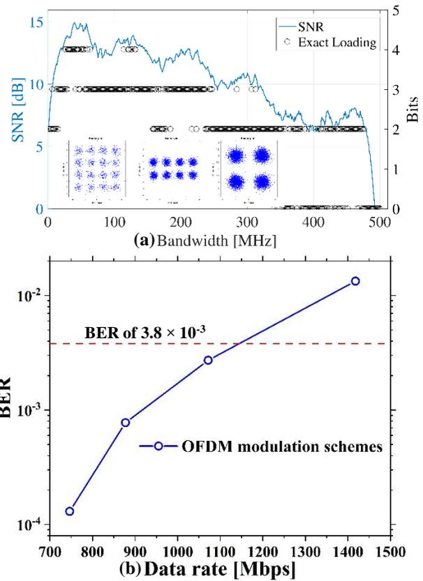
**Fig. 7.** (a) Measured SNR versus bandwidth for OFDM at  $J_{DC} = 1770$  A/cm<sup>2</sup> and  $V_{PP} = 7$  V.  $M$ -QAM constellation symbols received at the photodetector after equalization for  $M = 4, 8, 16$  are inserted; (b) data transmission rate versus BER for OFDM measurement at  $J_{DC} = 1770$  A/cm<sup>2</sup> and  $V_{PP} = 7$  V.
