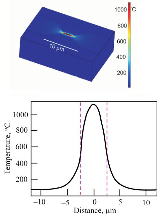
Fig. 2. The results of temperature modelling of a typical electrode geometry using COMSOL. In this example, a current of 14 mA was passed through the metal bridge and a temperature as high as 1000 °C was produced at the centre. The results illustrate the extremely high temperature gradients at the edge of the metal heater.
