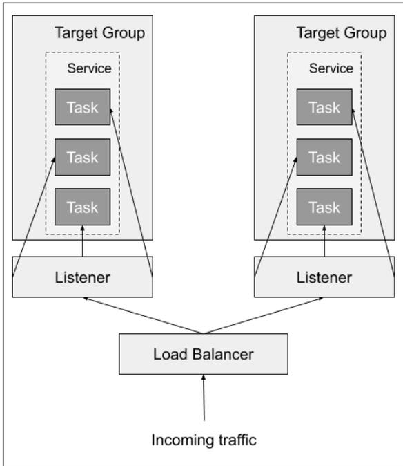
Figure 2: Routing traffic with a Load Balancer
