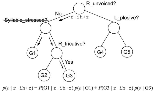
Figure 4: An example of decision tree marginalization, showing how a new recognition model “r-ih+z” is derived from a decision tree of a speech synthesis system (“L\_” / “R\_”: left/right phone; “G?”: clustered state emission distribution PDFs)
