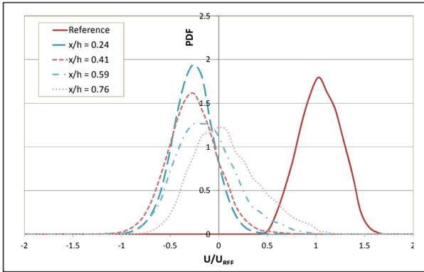
Figure 3. Probability density functions for the U velocity component at the reference anemometer and for four sonic anemometers lying alongside Taps V8-V11. The mean wind direction was  $86.5^\circ$ , almost perpendicular to the windward face.
