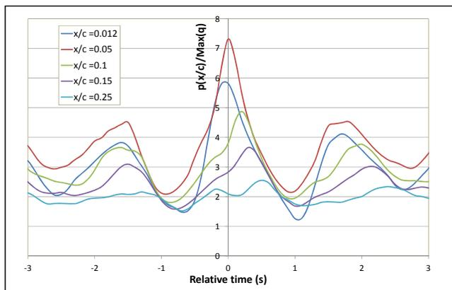
Figure 7. Conditionally averaged differential pressures on the 4/5<sup>th</sup> stripe. The trigger event used was the peak pressure at the second tap in the stripe ( $x/c=0.05$ ). The pressures were normalised using the maximum dynamic pressure recorded by the masthead anemometer within  $\pm 2s$  of the event.
