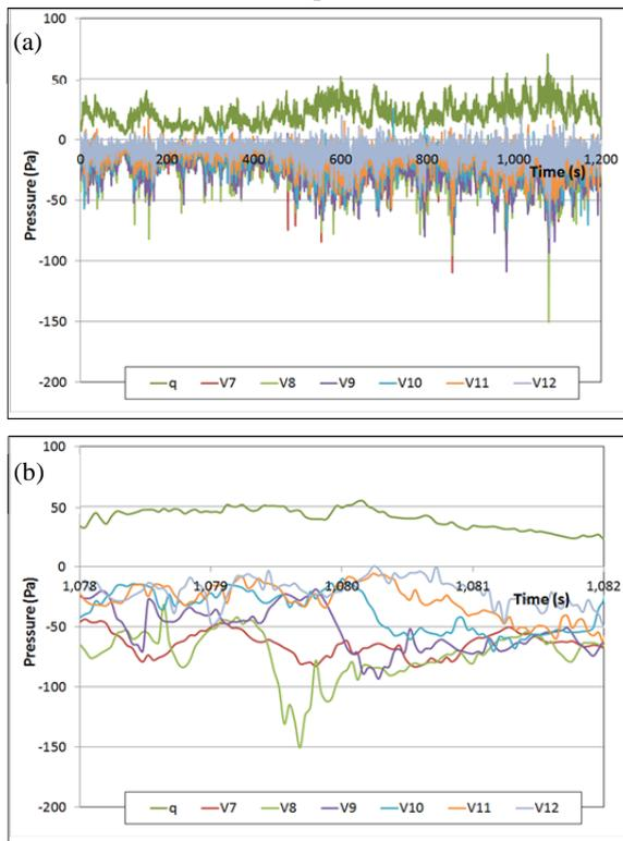
Figure 4. Full-scale pressure data from one 20 minute run during which the wind direction was  $\theta=86.5^\circ$ ; (a) time histories for the reference dynamic pressure  $q$  and the roof pressures, and (b) the same pressures expanded around the time of the lowest pressure which occurred at Tap V8 at a time of 1079.7s.
