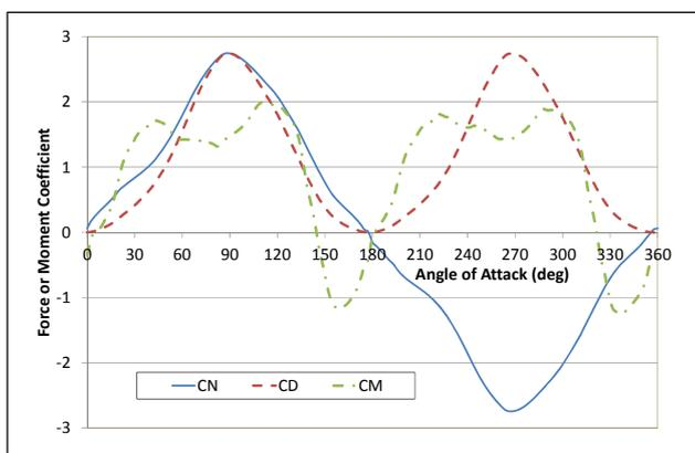
Figure 1. Normal force, drag force and pitching moment coefficients as a function of angle of attack determined by pressure integration. Wind speed 10 m/s.
