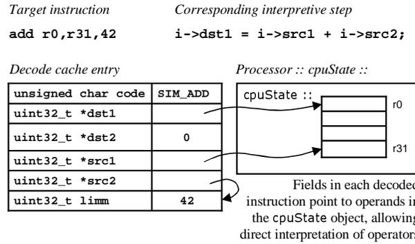
Fig. 3. Decode cache illustration and example add instruction.
