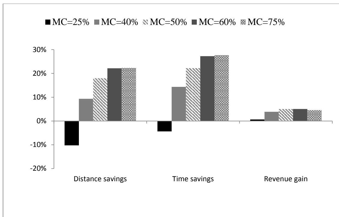
Figure 3 - Relative savings (compared to existing situation) for different minimum collection (MC) values
