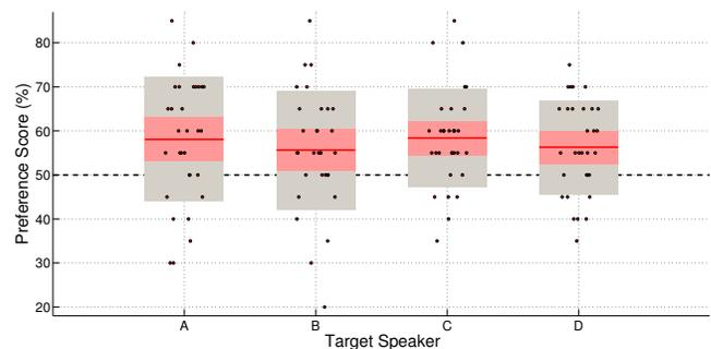
**Fig. 2.** Results of the listening test. Points representing average listeners preference score for each speaker (A, B, C, and D) are layed over a 1.96 standard error of the mean (SER) (95% confidence interval) in pink and a 1 standard deviation (SD) in grey.
