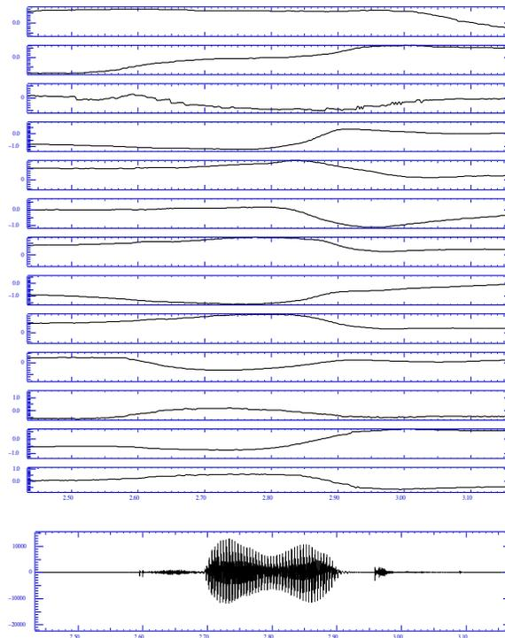
**Figure 1:** Example EMA data for the word “pod” . Tracks, reading from the top, are velum height (y), upper lip y, upper lip x, tongue tip y, tongue tip x, tongue dorsum y, tongue dorsum x, tongue blade y, tongue blade x, lower lip y, lower lip x, lower incisor y, lower incisor x. The y coordinate is vertical (increasing y means upward movement), and the x coordinate is horizontal (increasing x means forward movement).
