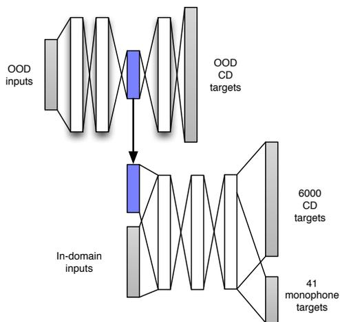
Fig. 2. Multitask network structure with MLAN features
