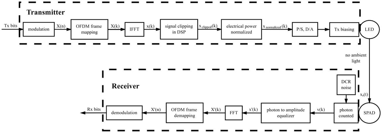
Fig. 1. Block diagram of the SPAD-based OFDM system.
