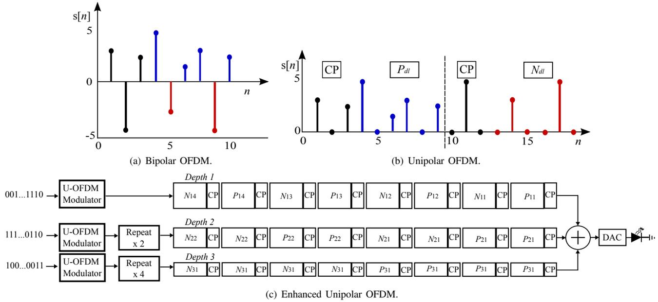
Fig. 1. Enhanced U-OFDM for a maximum modulation depth of 3. CP denotes the OFDM cyclic prefix in every frame.  $P_{dl}$  is the  $l$ th positive frame at Depth  $d$ .  $N_{dl}$  is the  $l$ th negative frame at Depth  $d$ . The presented digital-to-analog converter (DAC) block includes all processing techniques and electrical circuitry required for transition from a discrete-time-domain signal to a continuous analog signal capable of modulating the LED transmitter.
