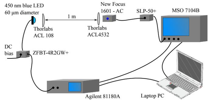
Fig. 9. Experimental set-up.
