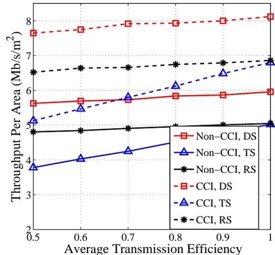
Fig. 12. Spatial throughput in non-CCI case and optical CCI case. (Wi-Fi throughput 1 Gb/s)
