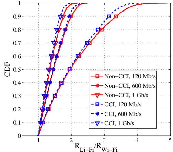
Fig. 9. CDF of the user data ratio  $R_{\text{Li-Fi}}/R_{\text{Wi-Fi}}$  in non-CCI and optical CCI case. The user density is set to be 0.2 person/m<sup>2</sup>, which is normal in the indoor office scenario. ( $\eta = 1$ )
