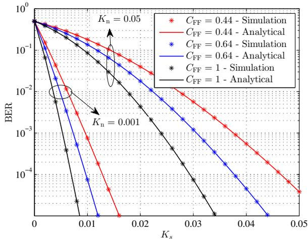
Figure 5. Analytical (solid curves) and simulation (asterisks) BER results of a  $64 \times 64$  SPAD array receiver for different values of  $C_{FF}$  and  $K_n$  ( $T_b = 1 \mu\text{s}$  and  $\tau = 1 \text{ ns}$ ).
