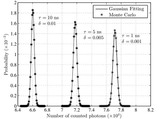
Figure 3. Probability distribution of a  $64 \times 64$  SPAD array photocounts for  $T_b = 1 \mu\text{s}$ ,  $\lambda = 3 \times 10^7$  photon/s,  $C_{\text{FF}} = 0.64$  and different values of  $\delta$ .
