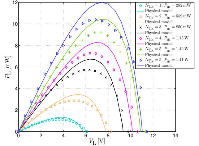
Fig. 4. Experimental  $V$ - $P$  curves of Study II.
