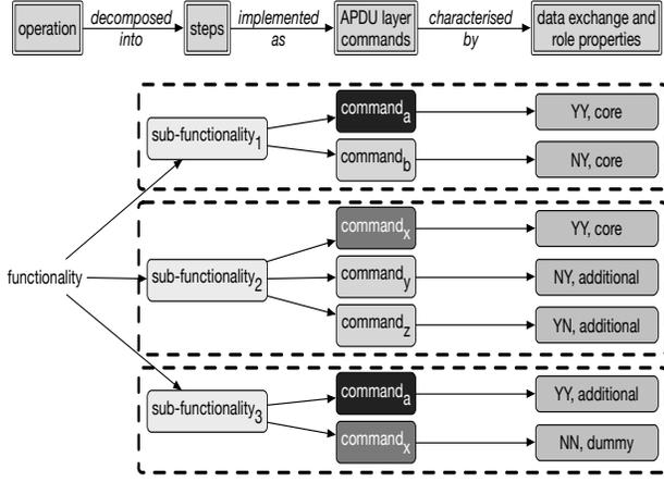
**Figure 3:** A single operation represents a specific functionality and it is modeled as a sequence of sub-functionalities. Each sub-functionality is further implemented as a sequence of commands. Commands are characterized by their data exchange properties and role within some particular sub-functionality.
