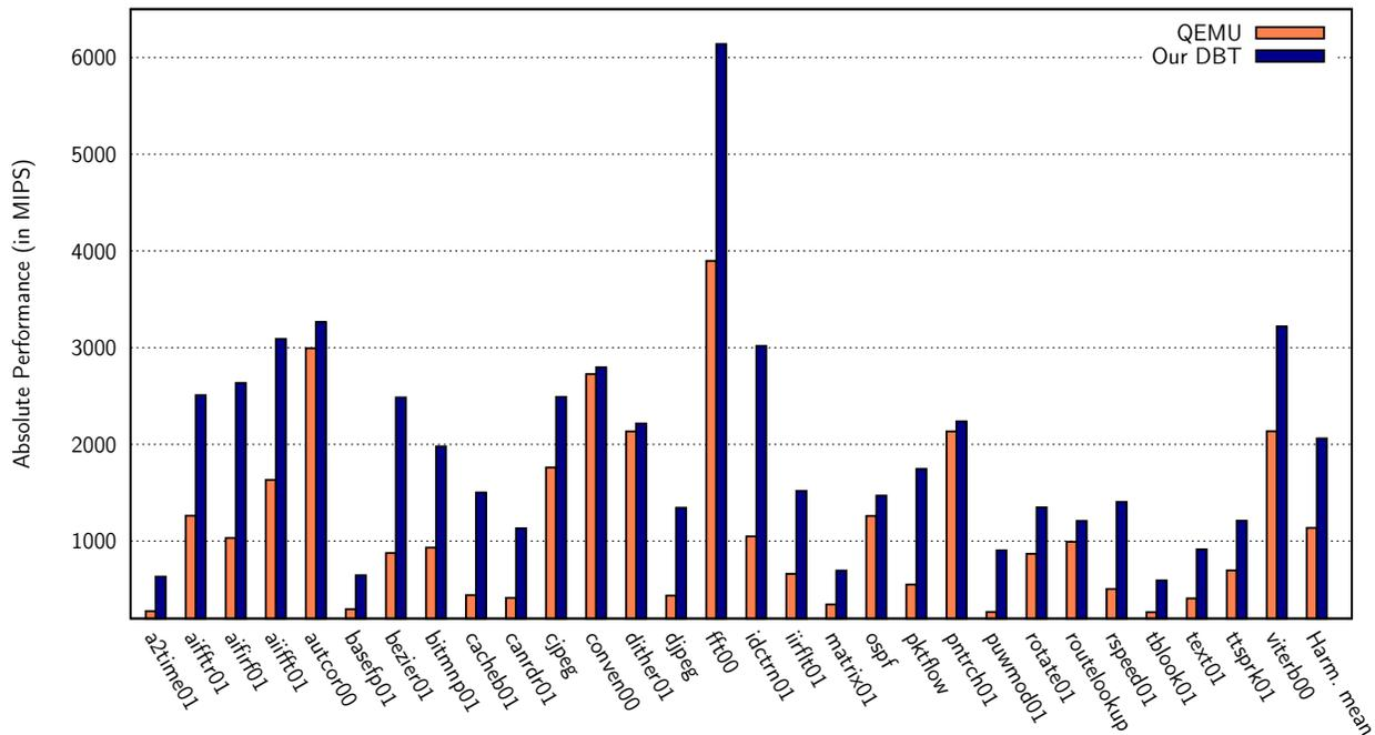
**Figure 9.** Absolute performance figures (in MIPS) for the *shorter-running* EEMBC benchmarks for both QEMU-ARM and our DBT, indicating that JIT startup time and compilation performance of our DBT is more than competitive with QEMU-ARM despite aggressive code optimisations applied by our system.
