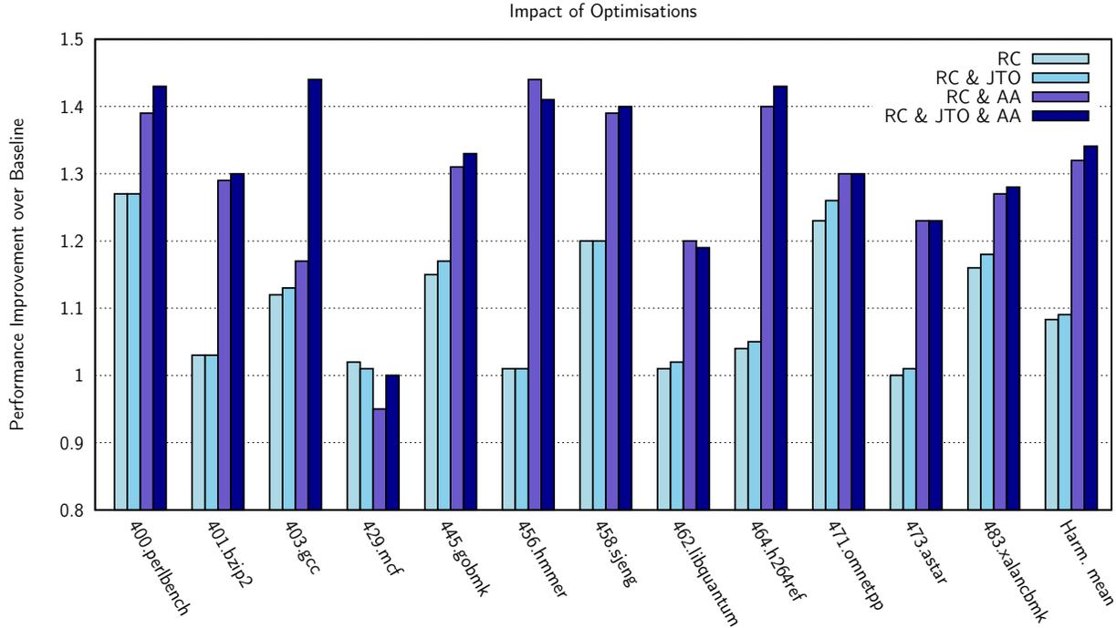
**Figure 8.** Breakdown of performance impact of different optimisations. Baseline is standard LLVM -O3 and partial evaluation (Wagstaff et al. 2013) at JIT compilation time. Additional region chaining (RC), jump table optimisation (JTO) and alias analysis (AA) complement each other.
