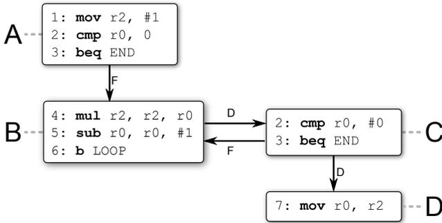
**Figure 1.** Blocks discovered by the profiler for the example code in Listing 1. An edge labelled **F** denotes a fall-through from a predicated branch, and an edge labelled **D** denotes a direct branch target.
