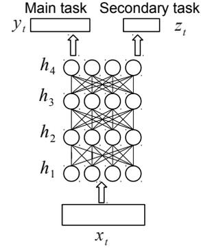
**Fig. 1.** A multi-task deep neural network (MTLDNN). In a MTLDNN, the main task and the secondary task share the same hidden representations (i.e., hidden layer activations). The optimisation criterion is to minimise the mean square error on both tasks.  $x_t$ ,  $y_t$  and  $z_t$  are the linguistic input, main task and secondary task, respectively, at frame  $t$ .  $h_k$  is the  $k^{\text{th}}$  hidden layer
