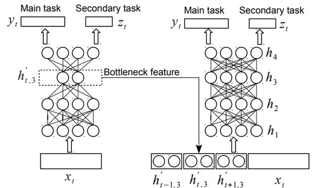
**Fig. 2.** Multi-task deep neural network (MTLDNN) with stacked bottleneck features. In this example, the bottleneck features for three consecutive frames are stacked as input to the second network. In practice, more than three frames can be included.  $h'_{t,3}$  is the vector of bottleneck feature for the  $t^{\text{th}}$  frame.
