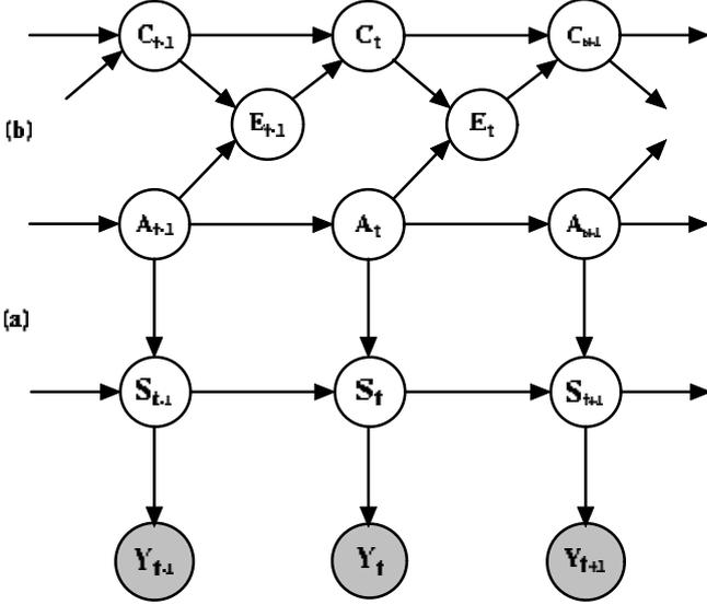
Fig. 1. Two-level HMM (a) with counter structure (b).
