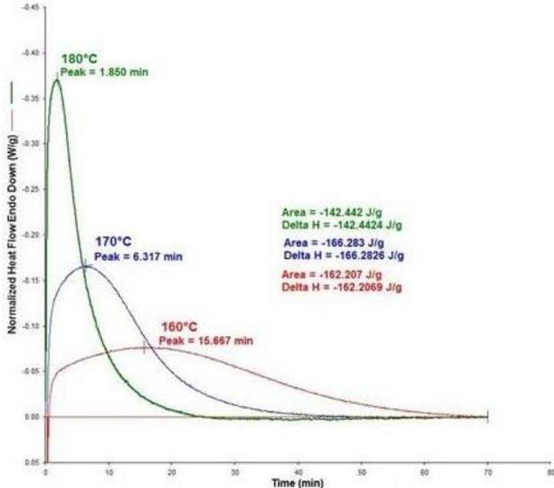
Fig. 4 Isothermal DSC curves at 3 cure temperatures
