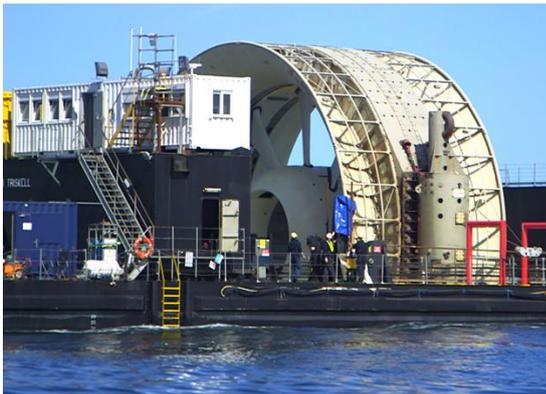
Fig. 1. OpenHydro's 16m Diameter Tidal Device
