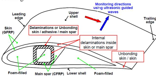
Fig. 7. SmartBlade Cut-away
