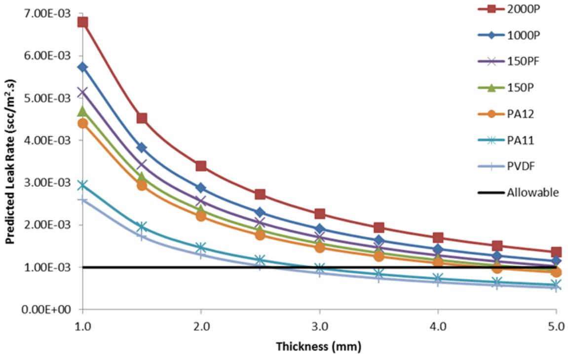
Fig. 7. Predicted leak rates for a 1 m<sup>2</sup> area of each material with a 5 bar pressure difference for varying liner thicknesses.
