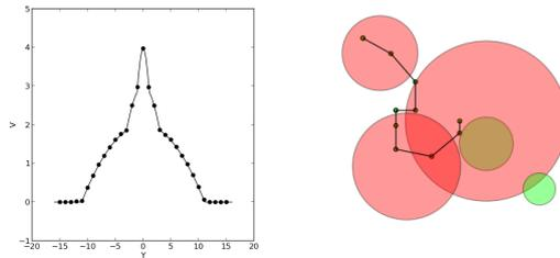
**Fig. 2.**  $V$ -function for different rover positions (with fixed  $X = 0.16$ ) in *simplerover1* domain (left). A possible episode in *marsrover* (right): each picture can be taken inside the respective circle (red if already taken, green otherwise).
