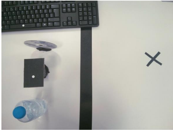
Fig. 4. Experimental environment. The three objects; the bottle, the card and the CD (numbered ‘1’, ‘2’ and ‘3’ respectively) are moved from their original position to the ‘X’ spot and the trial finishes.
