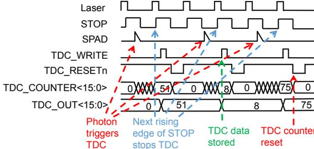
Fig. 4 TDC timing diagram in Histogram mode
