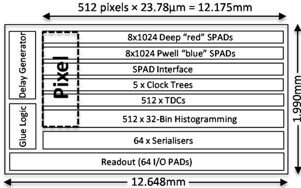
Fig. 2 Line sensor block diagram
