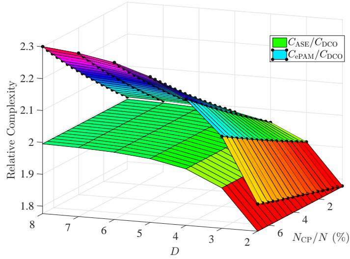
Fig. 5. The relative computation complexity of ASE-DMT and ePAM-DMT in comparison with the computation complexity of DCO-OFDM as a function of the total number of depths  $D$ , and the cyclic prefix percentage of the frame size  $N_{CP}/N$ .
