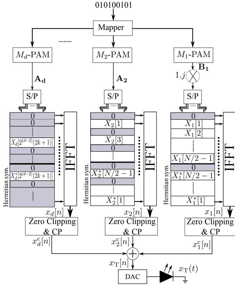
Fig. 1. ASE-DMT transmitter block diagram.  $X_d[k]$  refers to the  $k^{\text{th}}$  subcarrier at depth  $d$ ; S/P denotes for serial to parallel; DAC denotes for digital to analogue conversion; and CP refers to the cyclic prefixing.
