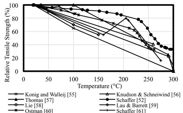
Figure 2: Tensile strength of timber as a function of temperature
