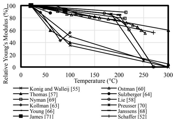
Figure 4: Modulus of elasticity of timber as a function of temperature
