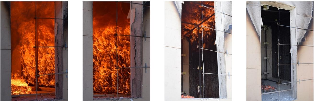
Progression to burnout and auto-extinction of a CLT wall following a compartment fire
