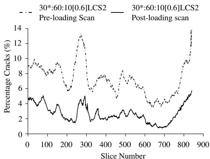
Figure 4: The area of cracks for each slice of 30\*:60:10[0.6] LCS2. Slice Number relates to depth below top surface of the sample, with slices spaced at 29.8 $\mu$ m.
