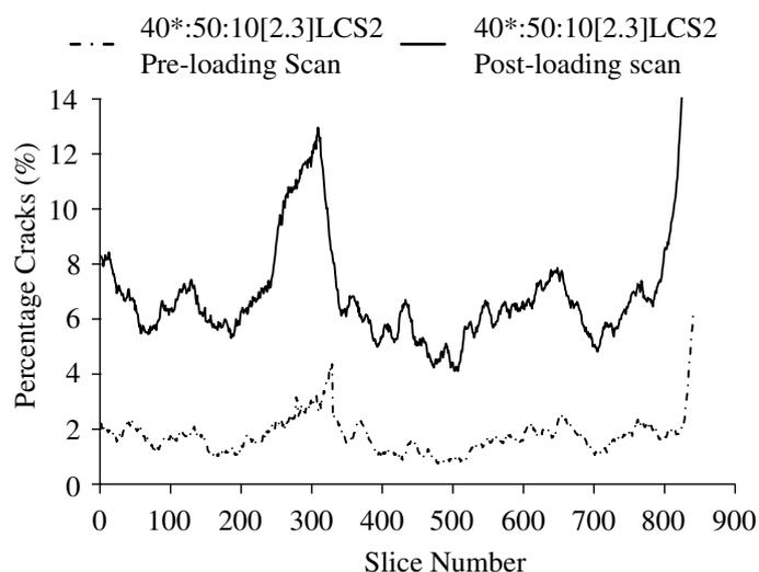
Figure 3: The area of cracks for each slice of 40\*:50:10[2.3] LCS2. Slice Number relates to depth below top surface of the sample, with slices spaced at 29.8 $\mu$ m.
