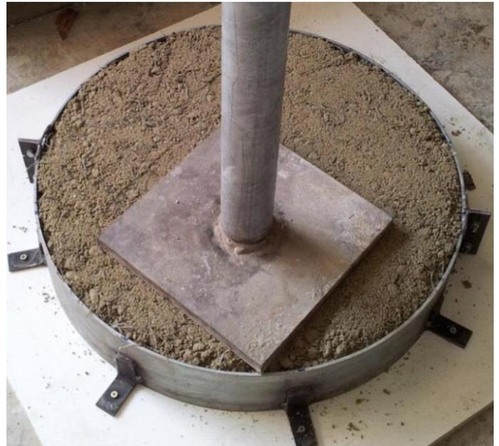
Figure 3. Initial manual compaction of specimen.
