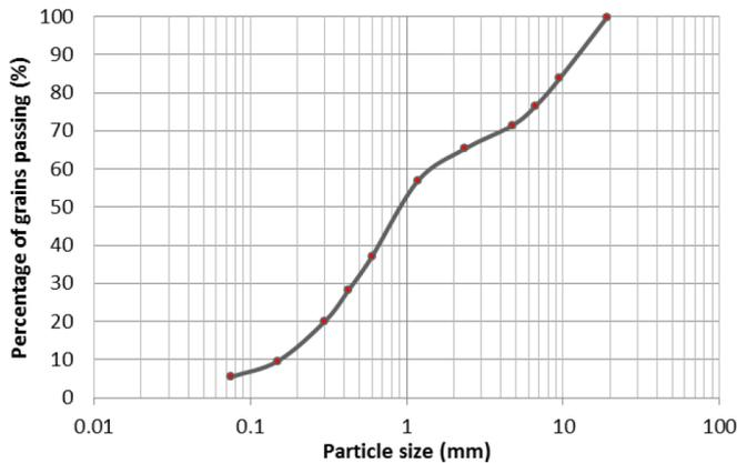
Figure 1. Particle size distribution of rammed earth mix.
