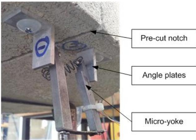
Figure 5. Positioning of micro-yoke and angle plates
