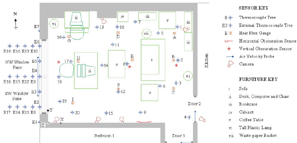
Figure 4: Test One: plan view of experimental compartment including furniture layout and fire sensor locations.
