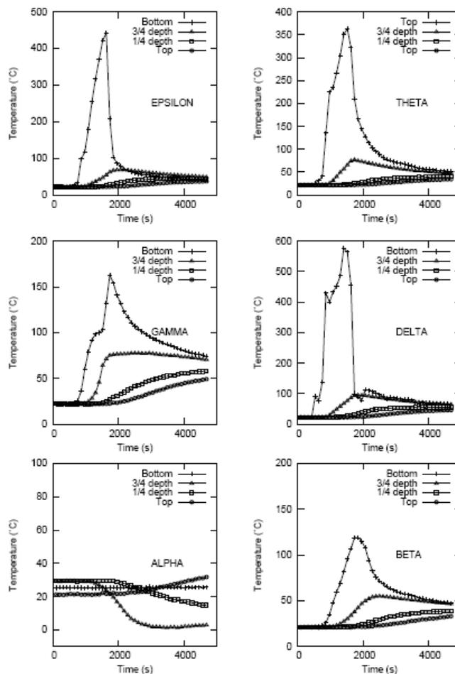
Figure 8: Thermocouple temperatures from the ceiling slab
