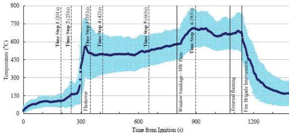
Figure 6: Gas-phase average compartment temperature-time curve variation with shaded regions indicating the standard deviation of temperature throughout the compartment
