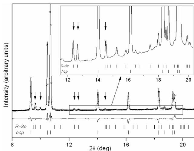
**Figure 2.** A two-phase *hcp*/*R* $\bar{3}c$  Rietveld refinement of Eu-III at 26.1 GPa. The experimental data are shown by the crosses and the fit by the solid line. The residuals are shown under the fit and the tick marks show the calculated peak positions. The arrows indicate the Eu-III reflections observed by Takemura and Syassen [1]. The inset shows an enlarged view of the high-angle part of the profile.
