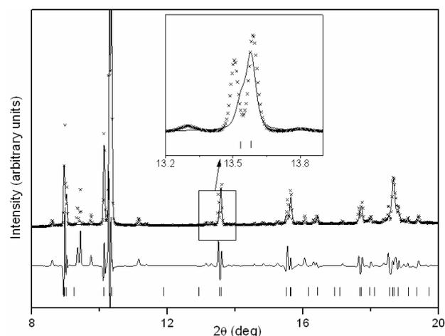
**Figure 4.** Le Bail refinement of a diffraction profile from a contaminant-free sample of Eu at 34 GPa, using the  $Pnma$  structure proposed by Bi *et al.* [5] for Eu above 41 GPa. The residuals are shown under the fit and the tick marks show the calculated peak positions. The inset shows an enlarged view of the fit to the split (102) peak from the *hcp* phase.
