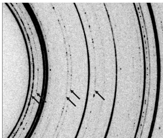
**Figure 1.** A 2D diffraction image from Eu at 26.1 GPa. The Debye-Scherrer (D-S) rings corresponding to the non-*hcp* reflections are spotty, whereas the *hcp* D-S rings are smooth. The arrows mark the five additional reflections observed by Takemura and Syassen [1].
