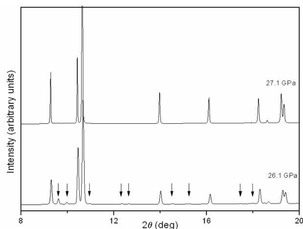
**Figure 3.** Integrated diffraction patterns from a contaminant-free sample of Eu at 27.1 GPa (upper) and a contaminated sample of Eu at 26.1 GPa (lower). Arrows in the lower profile mark the positions of the most intense  $R\bar{3}c$  peaks.
