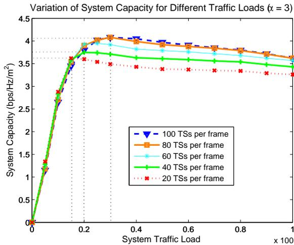
Fig. 3. Variation of system capacity with traffic loads for different TSs
