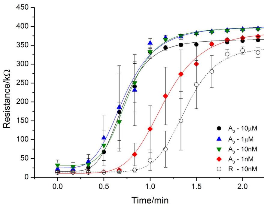
**Fig. 8.** The d.c. electrical response of carbon nanopowder OCPs swelling over time in analyte ( $A_0$ ) solutions of concentrations ranging from 10  $\mu\text{M}$  to 1 nM and a R solution of 10 nM. The solutions were held at 23  $^\circ\text{C}$  and contained 150 mM NaCl and 1 mM phosphate buffer.
