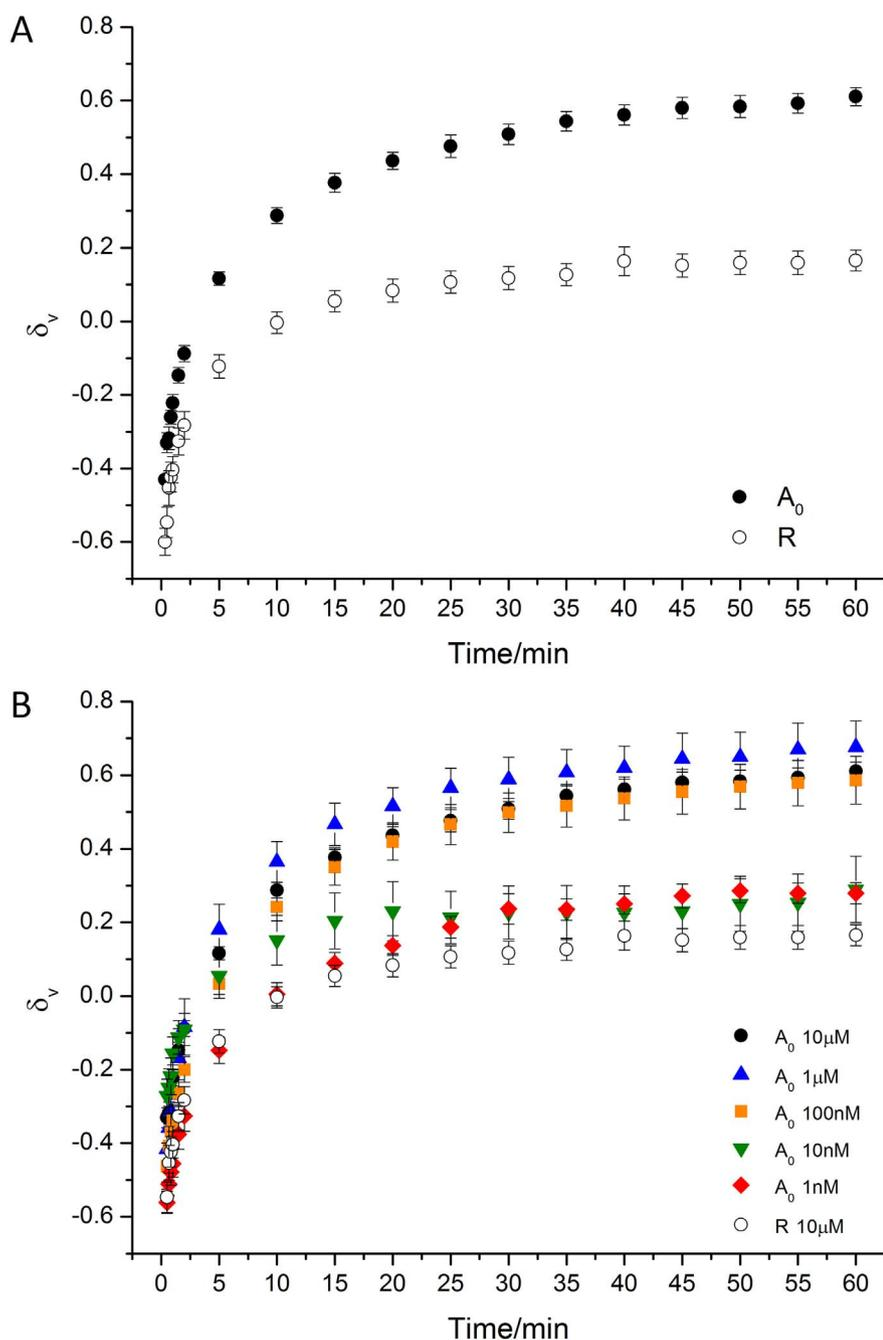
Fig. 4. A: Fractional volume increase with time for oligonucleotide-functionalised composites in  $A_0$  and R solutions of 10  $\mu\text{M}$ , B: Fractional volume increase against time for oligonucleotide-functionalised composites in solutions of varying  $A_0$  concentration and R solution of 10  $\mu\text{M}$ . All solutions were held at 23  $^{\circ}\text{C}$ .
