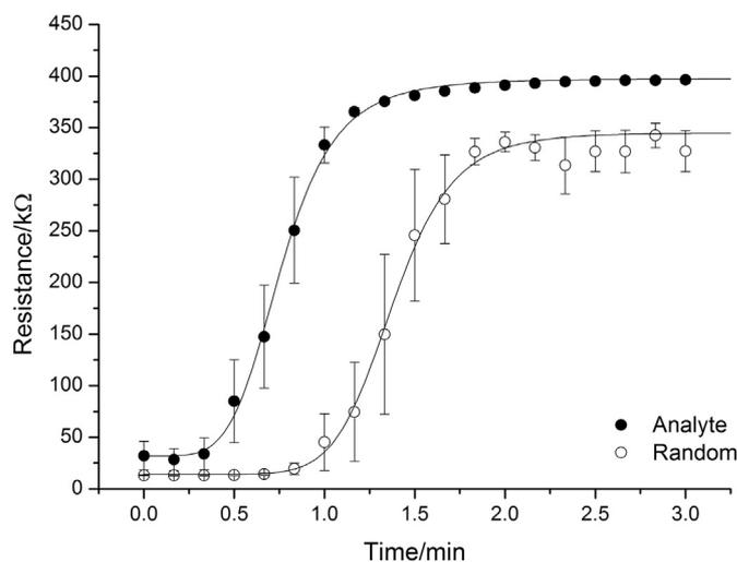
Fig. 7. The d.c. electrical response of OCPCs swelling over time in 10 nM  $A_0$  and R solutions. The solutions were held at 23  $^{\circ}\text{C}$  and contained 150 mM NaCl and 1 mM phosphate buffer.
