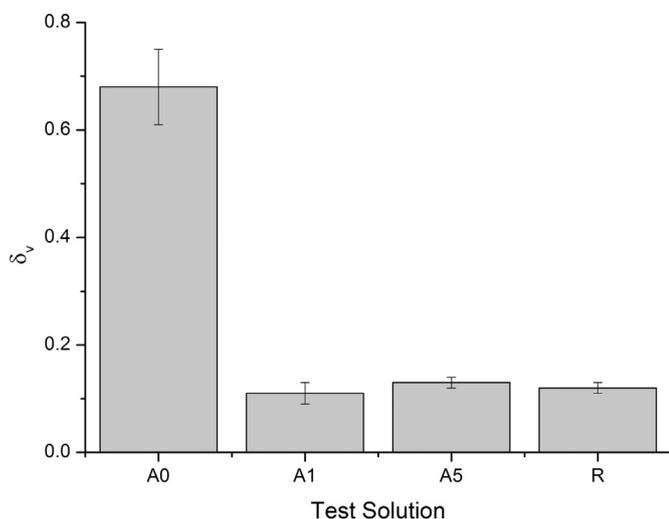
Fig. 5. The fractional volume increase for OCPCs in various oligonucleotide solutions. The solutions contain 1  $\mu\text{M}$  of either a perfectly complementary analyte sequence ( $A_0$ ), a single-mismatch sequence ( $A_1$ ), a five-mismatch sequence ( $A_5$ ) or a random sequence (R). All solutions contain 150 mM NaCl and 1 mM phosphate buffer. All solutions were held at 23  $^{\circ}\text{C}$ .
