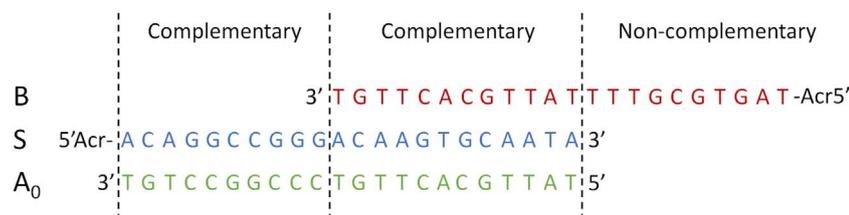
Fig. 2. The sequences and respective complementarity of the S, B and A<sub>0</sub> oligonucleotide sequences. 'Acr' denotes the acrydite modifier. The vertical dashed lines delineate the respective regions of complementarity.
