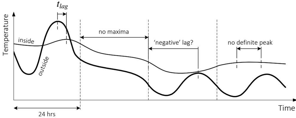
Figure 6: Filtering processes used to define thermal lag
