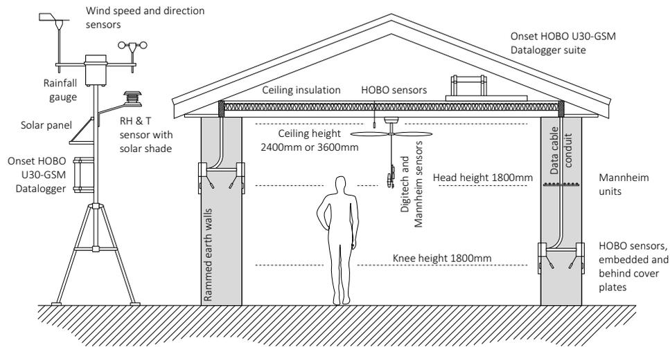
Figure 3: Diagrammatic representation of instrumentation locations. RH & T: Relative humidity and temperature (dry bulb)
