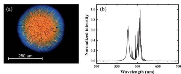
**Fig. 2** Results from inkjet deposition on to a cleaned, untreated glass substrate: (a) the deposited drop profile, between crossed polarizers, showing considerable non-uniformity; (b) the multimode emission spectrum under optical excitation at a wavelength of 532 nm.
