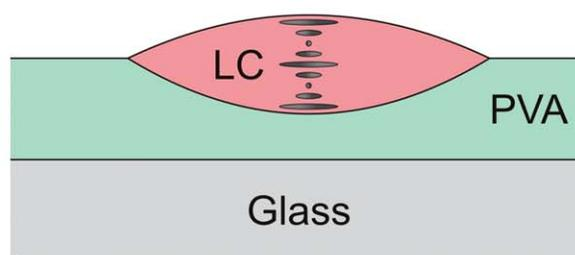
**Fig. 4** High-speed camera images of the droplet impact process (left) and pictorial representation of the sample cross-section (right) with the chiral LC in the Grandjean, or standing helix, alignment.
