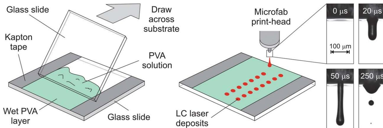
**Fig. 1** Schematic of the jetting and deposition process used in the work showing (left) creation of the wet polymer (PVA) solution, deposition of lasing LC media (middle) and (right) dynamics of the inkjet droplet formation from the printhead.
