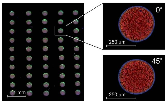
**Fig. 3** Pictures of inkjet printed LC laser droplets on a PVA film; (left) a regular array of droplets; (right) close up images (between crossed polarizers) of deposited droplets showing the rotationally invariant texture.
