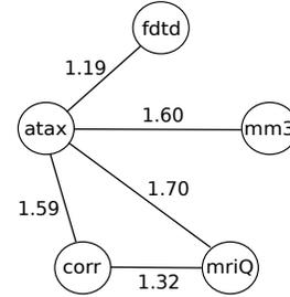
**Figure 2.** The task co-execution graph  $G = (V, E, w)$  describes the benefits we can expect from co-execution. A node  $V$  represents a kernel; an edge  $E$  links two nodes if their co-execution performs better than sequential run; the weight  $w$  of each edge quantifies the benefit.
