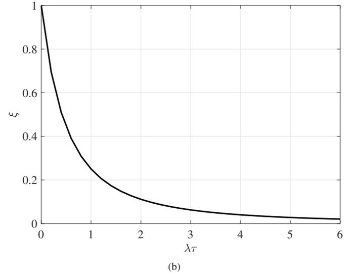
Fig. 2. First and second moments of AQ SPAD photocounts with  $T_b = 1 \mu\text{s}$ ,  $\tau = 2 \text{ ns}$ : (a) comparison of mean and variance with ideal Poisson distribution, (b) the variance to mean ratio.
