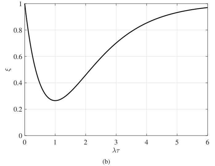
Fig. 4. First and second moments of PQ SPAD photocounts with  $T_b = 1 \mu\text{s}$ ,  $\tau = 2 \text{ ns}$ : (a) comparison of mean and variance with ideal Poisson distribution, (b) the variance to mean ratio.
