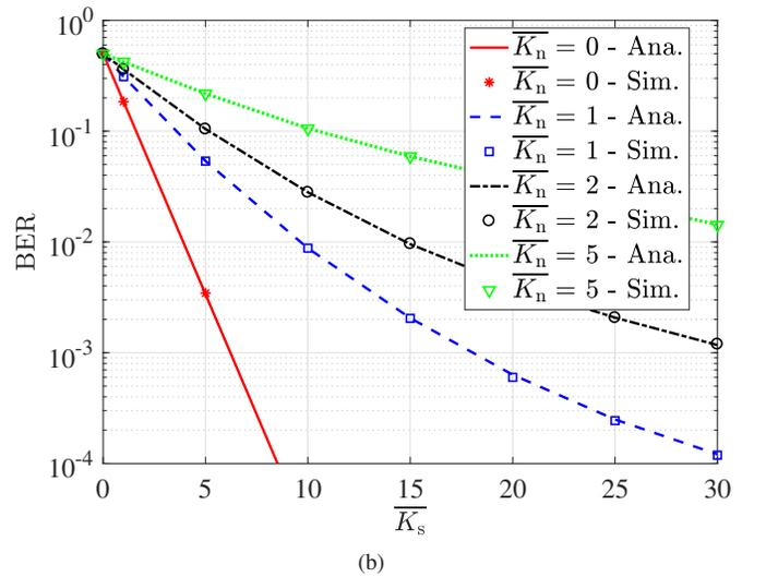
Fig. 5. OOK bit error performance of an AQ SPAD-based system: (a)  $\delta = 0.01, 0.001$  and (b)  $\delta = 0.1$ .
